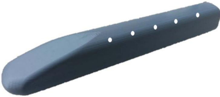
Fig. 29: Model of train with installed sensors
