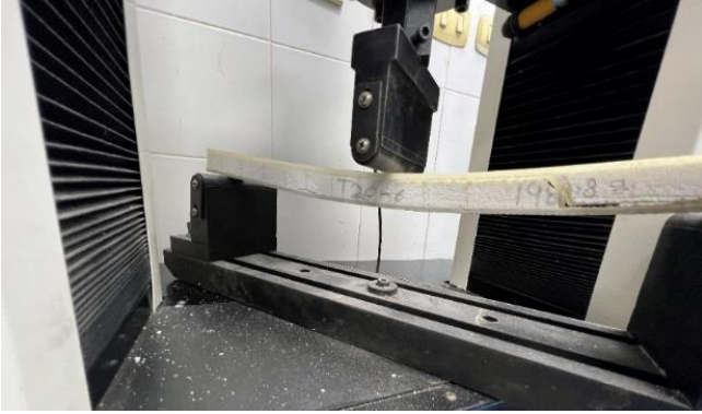
Fig. 4: the core shear failure on T20
