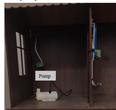
Fig. 6 Fire detecting system and the water pump
