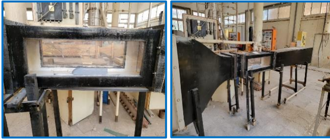
Fig. 15: Wind tunnel and the test section.
