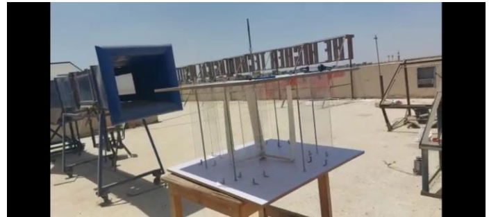
Fig. 7 Turbine test using wind tunnel
