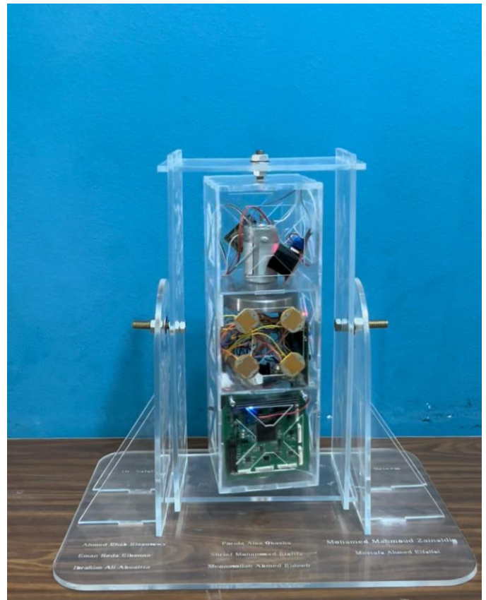
Fig. 8 The fabricated 3u form CubeSat structure assembling the overall system parts.
