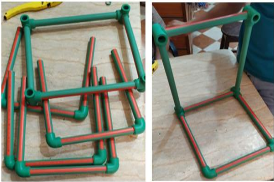
Fig 1 Cutting and joining the PVC
