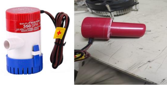
Fig 3 Bilge Pump before and after cutting
