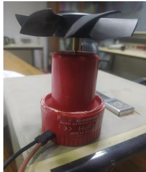
Fig 4 Modified thruster with propeller
