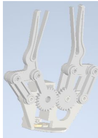
Fig. 8 the end effector or gripper of the robot arm
