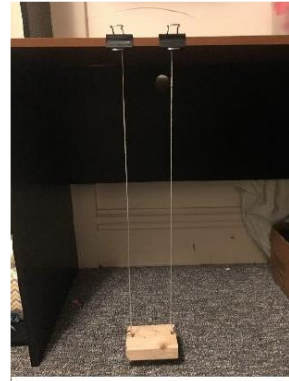
Figure 6: Setup to determine the moment of inertia about the y-axis
