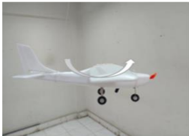
Figure 7(c) I yy measurement.
