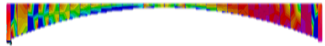
Fig. (1): The resultant stresses analysis of HCB repeated bay by Sap2000 software
