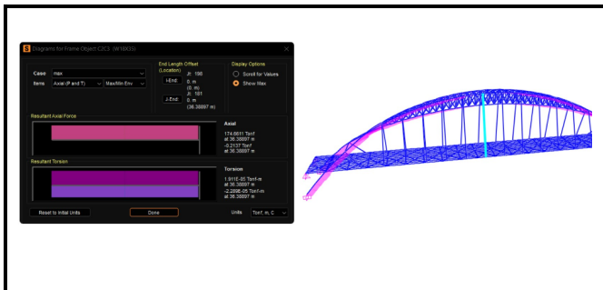
Figure 14 hanger axial force vertical arrangement)
