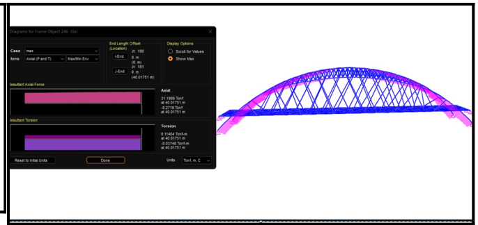
Figure 16 hanger axial force (Network arrangement)
