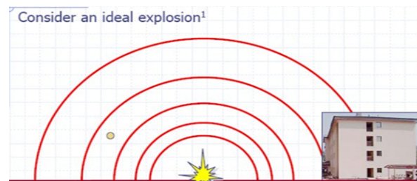
Fig. 1 a) Ideal free field blast wave profile[8]
