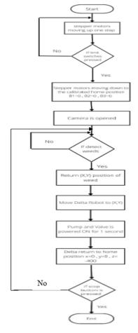
Figure 11: Integration of the Three Steps Algorithm
