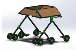
Figure 2: Rocker-Bogie Mechanism
