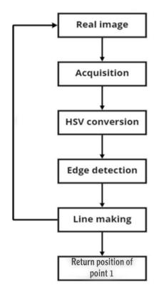
Figure 5: Computer Vision and Image Processing Algorithm
