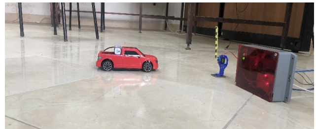
Figure (6). Gate is open and green light is ON at distance < 50 cm
