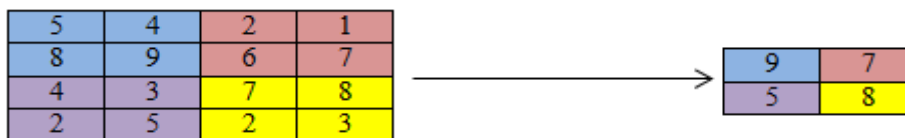
Figure 1 :Max Pooling using 2 \times 2 filter and stride 2.
