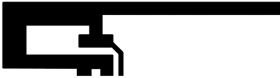
Fig. 5 Typical 2.4GHz Inverted F antenna.
