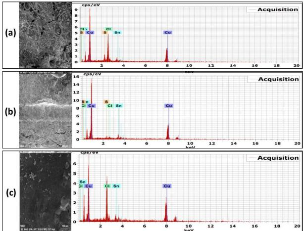
Figure 3 (a) shows the SEM & EDS of sample (1) and pitting corrosion appears well, (b) shows the SEM & EDS of sample (2) from the axe with rough surface, (c)shows the SEM & EDS of sample (3) surface with chloride impurities.
