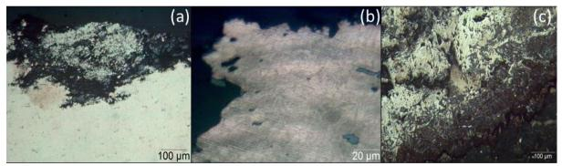
Figure 2 shows a metal sample from the axe using a metallographic microscope, (a) localized corrosion on the surface of axe, (b) the structure of the axe and pitting corrosion, (c) deep cracks inside the sample.
