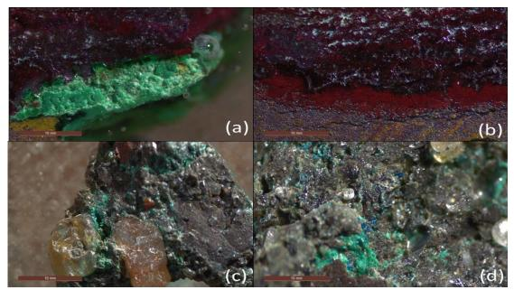
Figure 1 shows samples of corrosion products using optical microscope, (a) Paratacamite in a chalky green color, and Wustite (FeO) in a dark yellow color, (b) succession of layers of corrosion products in the sample and the presence of a layer of red iron impurities, (c-d) the overlapping of soil sediments with the Brochantite compound, which has a green color, and is produced due to the presence of sulfates.
