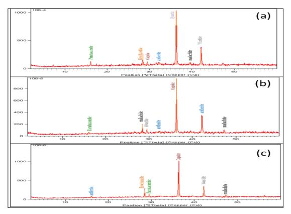
Figure 4 shows an X-ray diffraction analysis of the three samples, (a) the first sample, (b) the second sample, (c) the third sample, and the patterns of samples show approximately the same corrosion products.
