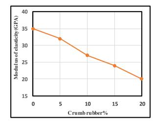
Fig. 7. Elastic modulus for various mixes
