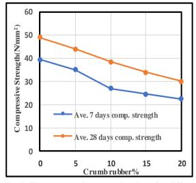
Fig. 2. The compressive strength values for different mixes
