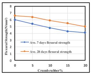
Fig. 3. The flexural strength values for different mixes
