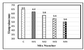
Fig. 1. Slump values for various mixes
