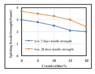
Fig. 4. The splitting tensile strength values for different mixes
