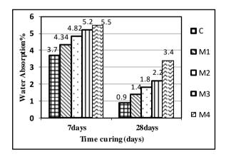
Fig. 5. The rate of water absorption values for various mixes
