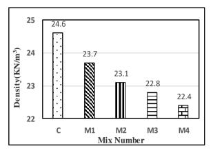
Fig. 6. Density values for different mixtures at 28 days of curing
