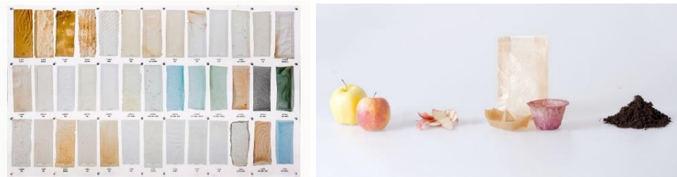
Figure 9 : On the right: Shellworks has made bioplastic chitosan a viable alternative of many plastics in use (Girard, T., 2019) On the left: bioplastic chitosan has variable colors and translucency. (Girard, T., 2019)
