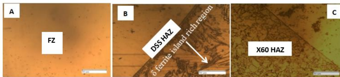
Fig. 9 Microstructures of FZ and HAZ at medium heat input welding condition: (a) FZ, (b) DSS HAZ with \delta ferrite island rich region and (c) X60 HAZ
