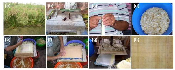
**Fig. 2.** Commercial papyrus manufacture at Qaramos, Egypt. (a) Papyrus plants ready for cultivation; (b) Cutting the stems using an electrical cutter; (c) Slicing the papyrus stem into strips with a nylon thread; (d) Soaking papyrus strips in a dilute sodium hydroxide solution; (e) Layering the strips into orthogonal layers; (f) Placing papyrus sheets between linen and cardboard; (g) Pressing papyrus sheets using a manual press; (h) A final papyrus sheet.
