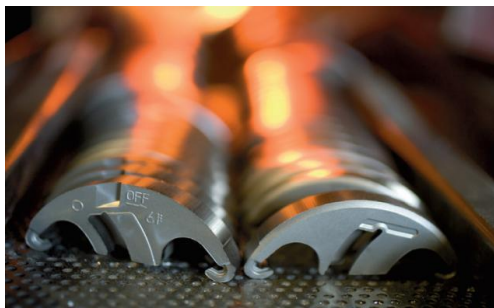
Fig. 6 Sintering of compacted tool steel parts.
