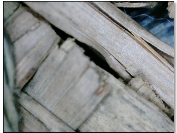
Shape (10) shows the detachment of fiber (zoom
