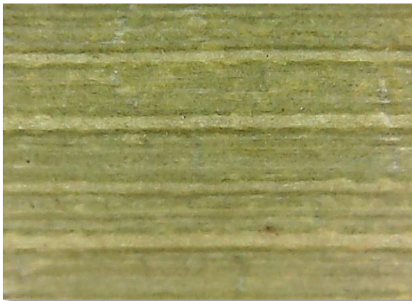
Shape (14) shows the surface appearance of the brush sample, where there are longitudinal fiber cracks (zoom force of 10000X).
