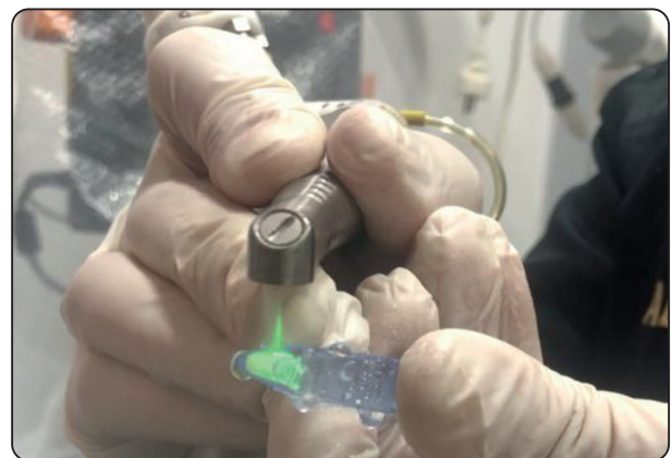
Fig. (2): Zirconia specimens treated with Er:YAG laser
