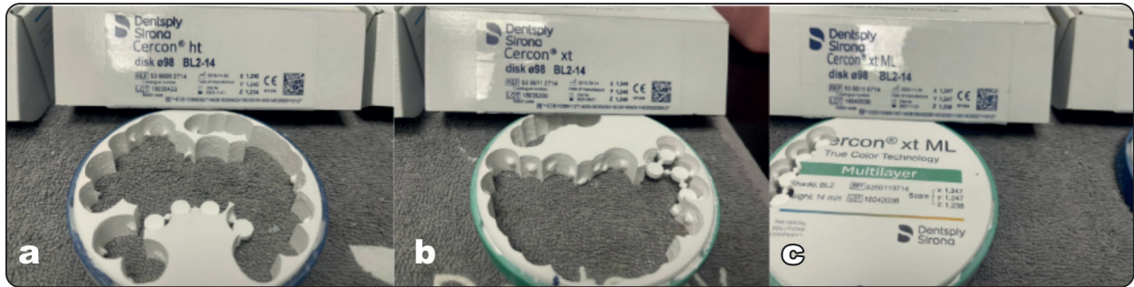
Fig. (1): The three types of Zirconia discs (a. For translucent zirconia b. High translucent zirconia c. Ultra translucent zirconia).
