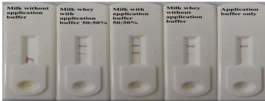
Fig. (2): Effect of methods of milk samples preparation on the Test results of the lateral flow procedure ( E. coli LFD).
