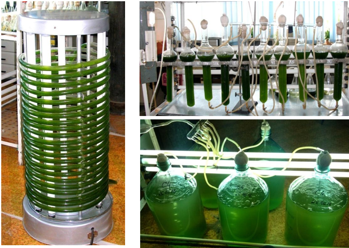
Fig.1. Bioreactors for the cultivation of microalgae in closed controlled conditions
