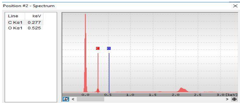
Fig. 3. EDX-analysis for Poly-urethane foam
