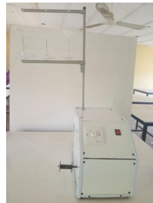
Figure 6: The Complete View of Fabricated Electric Yarn Winder for Hand Woven Fabric Production. Source: Researcher's fieldwork (2022)
