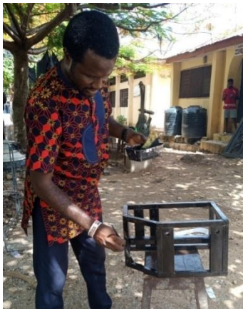
Plate 3: Painting of the machine frame to prevent rust Source: The Researcher's fieldwork (2022)
