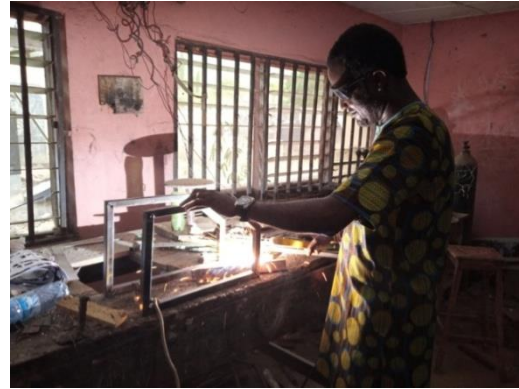
Plate 2: Welding the pipes together to form the machine frame Source: The Researcher's fieldwork (2022)
