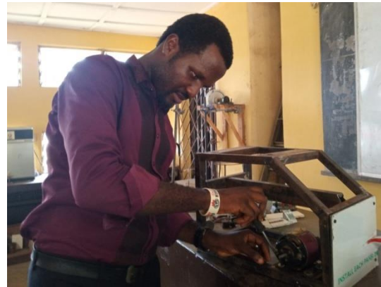
Plate 4: Fastening the electric Motor unto the frame of the machine. Source: The Researcher's fieldwork (2022)
