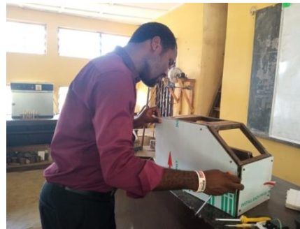
Plate 8: Setting and fixing of the Alco-board on the fabricated electric yarn winder.
