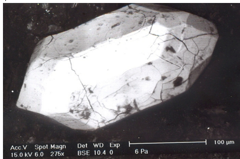
Fig.16: EDX and BSE image of metamict zircon
