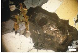
Fig.6: Photomicrograph showing chloritized biotite protruded the zoned saussuritized plagioclase in monzogranite, XPL
