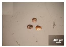
Fig.44: Hematite grains from altered monzogranite
