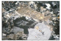
Fig. 11: Photomicrograph showing a graphic texture and plagioclase alteration to epidote in altered monzogranite, XPL
