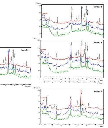
Fig.3: Examples of the X-ray diffraction patterns of the variegated and black shale samples in Sibaiya area, West Nile Valley
