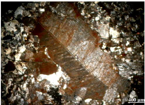
Fig.13: Photomicrograph of euhedral crystal of feather perthite coated by iron oxides in syenogranite, XPL
