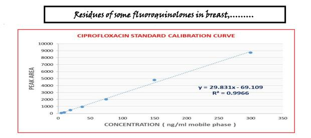
Fig. (4): Matrix matched standard calibration curve of ciprofloxacin for kidney extract dissolved in mobile phase (Coefficient of Determination, R2=0.9966).
