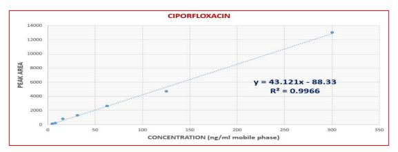
Fig. (5): Matrix matched standard calibration curve of ciprofloxacin for liver extract dissolved in mobile phase (Coefficient of Determination, R2=0.9966).
