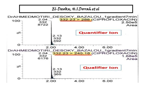
Fig. (2): Representative chromatogram showing quantifier and qualifier ions of ciprofloxacin as generated by the Quanpedia software and confirmed by the experimental work.
