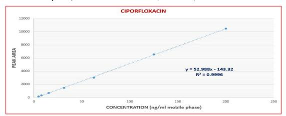
Fig. (6): Matrix matched standard calibration curve of ciprofloxacin for muscles extract dissolved in mobile phase (Coefficient of Determination, R2=0.9996).
