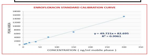
Fig. (7): Matrix matched standard calibration curve of enrofloxacin for kidney matrix dissolved in mobile phase (Coefficient of Determination, R2=0.9961).
