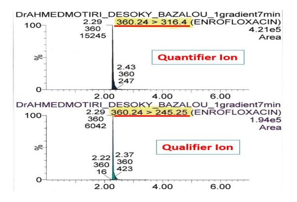
Fig. (3): Representative chromatogram showing quantifier and qualifier ions of enrofloxacin as generated by the Quanpedia software and confirmed by the experimental work.
