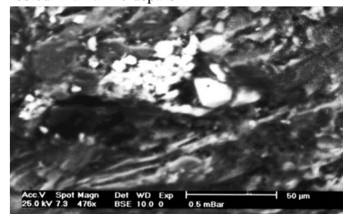
Fig. 9: BSE image of native silver aggregates (bright colour) occurs as inclusions within chalcopyrite (dark)
