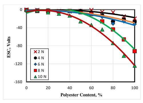
Fig. 11 ESC generated on the surface of cotton/PET blended by carbon fibers from the sliding on wool.
