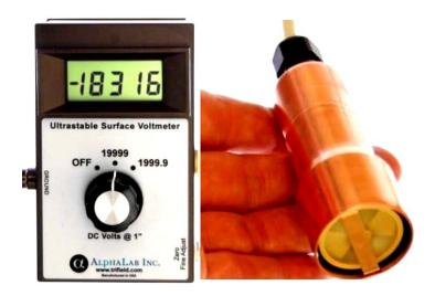
Fig. 2 Electrostatic field measuring device.
