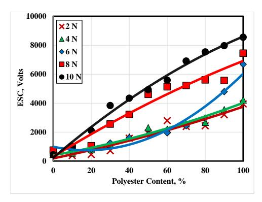
Fig. 5 ESC generated on the surface of wool from the contact-separation with cotton/PET.
