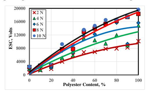
Fig. 7 ESC generated on the surface of wool from the sliding on cotton/PET.
