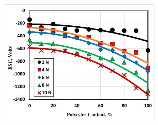
Fig. 4 ESC generated on the surface of cotton/PET from the contact-separation with wool.
