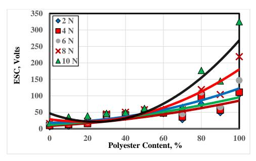
Fig. 10 ESC generated on the surface of wool from the contact-separation with cotton/PET blended by carbon fibers.
