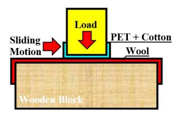
Fig. 3 Arrangement of the test procedure.
