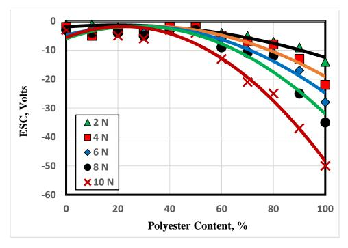
Fig. 9 ESC generated on the surface of cotton/PET blended by carbon fibers from the contact-separation with wool.
