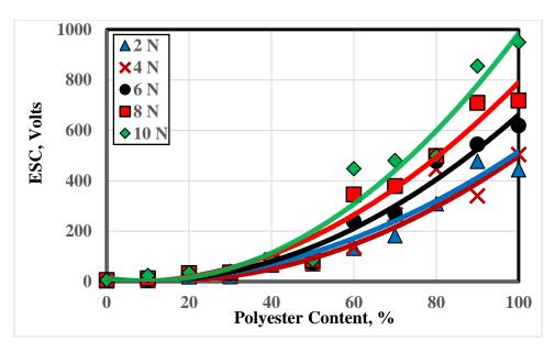
Fig. 12 ESC generated on the surface of wool from the contact-separation the sliding on cotton/PET blended by carbon fibers.
