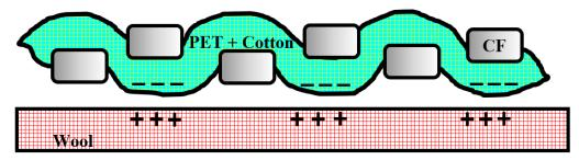
Fig. 8 Representation of ESC generated on the contact surfaces; after contactseparation and sliding.
