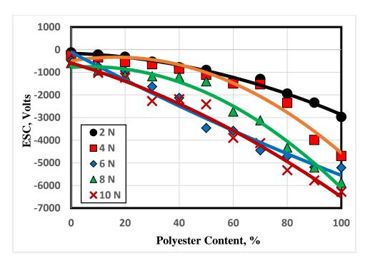
Fig. 6 ESC generated on the surface of cotton/PET from the sliding on wool.
