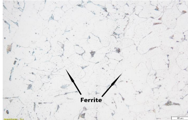
Fig. 9 Microstructure of low forging and friction pressure with a coarse ferrite grain.
