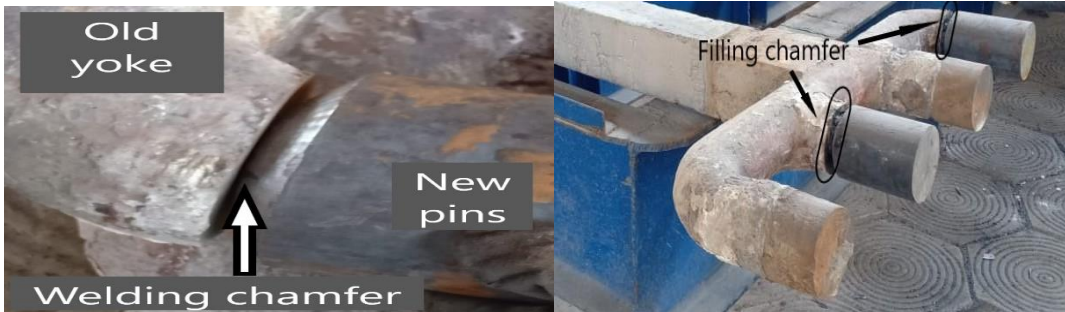
Fig. 5 Chamfer of the traditional fusion welding.
