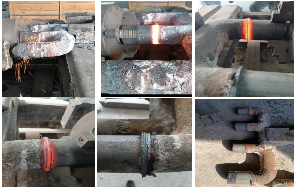
Fig. 3 Yoke welding process stages.
