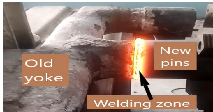
Fig. 6 Complete diffusion during friction welding.
