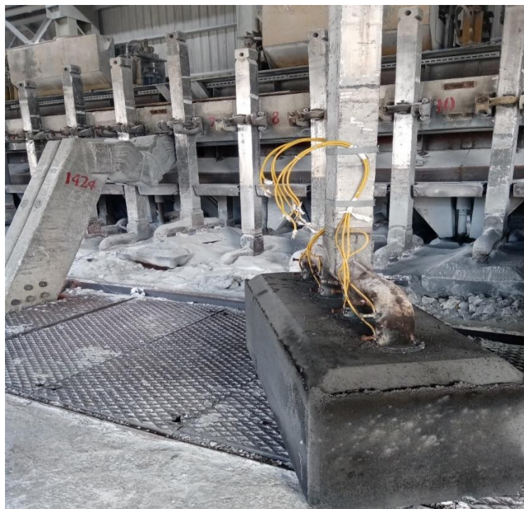
Fig. 4 The complete anodic conductor.
