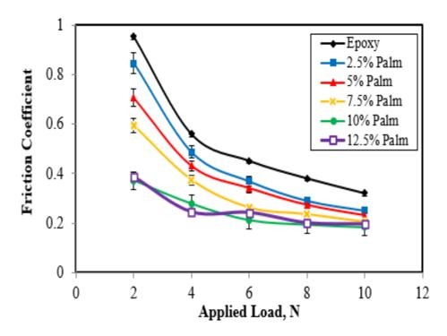
Fig. 8 COF of epoxy resin filled with different filler content palm oil.
