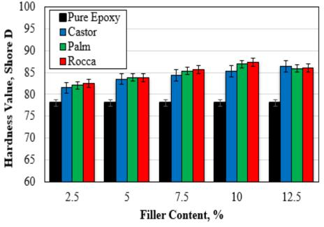
Fig. 6 Hardness shore D values of epoxy resin filled with different type natural oils.
