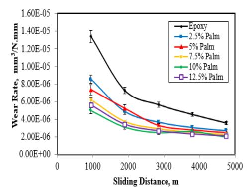
Fig. 12 Wear rate of epoxy resin filled with different filler content palm oil.
