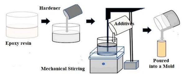
Fig. 1 Schematic diagram of epoxy sample preparation.
