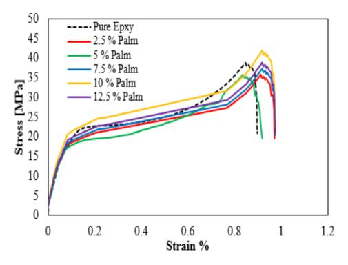
Fig. 4 Stress strain curve of epoxy resin filled with different filler content palm oil.
