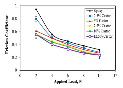
Fig. 7 COF of epoxy resin filled with different filler content castor oil.
