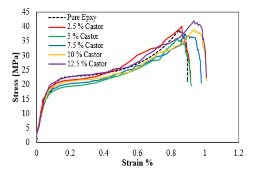
Fig. 3 Stress strain curve of epoxy resin filled with different filler content castor oil.
