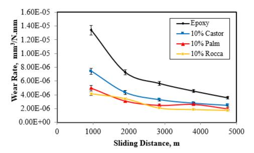
Fig. 14 Comparison of Wear rate between epoxy resin filled with different oils.
