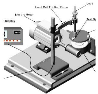
Fig. 2 Arrangement of tribometer test rig.
