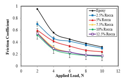
Figure 9 COF of epoxy resin filled with different filler content rocca oil.
