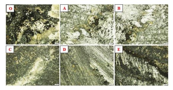
Fig. 16 Optical topography images of epoxy matrix filled with palm oil, (O) free epoxy matrix, (A) 2.5 % palm oil, (B) 5 % palm oil, (C) 7.5 % palm oil, (D) 10% palm oil, and (E) 12.5 % palm oil.
