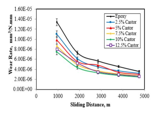
Fig. 11 Wear rate of epoxy resin filled with different filler content castor oil.
