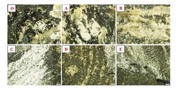
Fig. 17 Optical topography images of epoxy matrix filled with rocca oil, (O) free epoxy matrix, (A) 2.5 % rocca oil, (B) 5 % rocca oil, (C) 7.5 % rocca oil, (D) 10% rocca oil, and (E) 12.5 % rocca oil.
