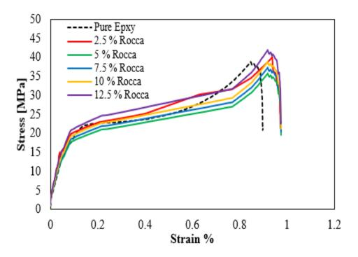
Fig. 5 Stress strain curve of epoxy resin filled with different filler content rocca oil.
