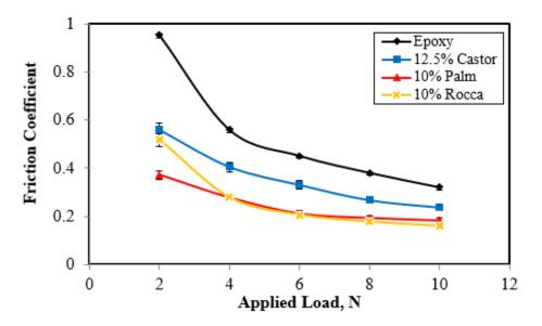
Fig. 10 Comparison of COF between epoxy resin filled with different oils.
