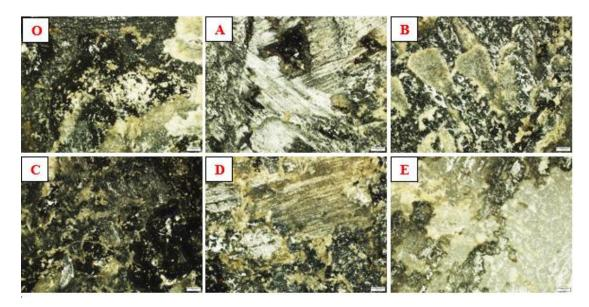
Fig. 15 Optical topography images of epoxy matrix filled with castor oil, (O) free epoxy matrix, (A) 2.5 % castor oil, (B) 5 % castor oil, (C) 7.5 % castor oil, (D) 10 % castor oil, and (E) 12.5 % castor oil.
