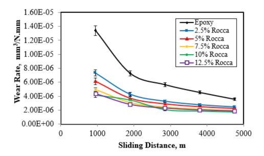
Fig. 13 Wear rate of epoxy resin filled with different filler content rocca oil.
