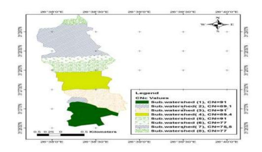
Figure (5): The Composite Curve Numbers (CNc) of the sub watersheds of wadi Shebity
