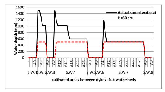
Figure (8): The depth of Stored Water /Water depth required for Cultivated Areas
