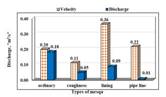
**Fig. 8.** Effect of modernized surface irrigation system on velocity and discharge.
