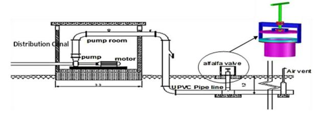
Fig. 4. Vertical section for buried pipelines.
