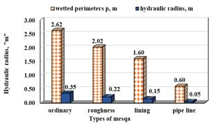
**Fig. 9.** Effect of modernized surface irrigation system on hydraulic radius and wetted perimeters.
