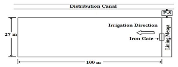
Fig.1. General layout of modernized surface irrigation (lining mesqa) for field (No.1)
