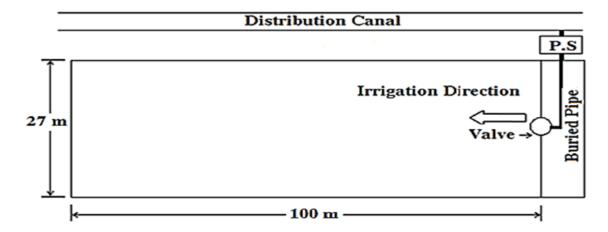
Fig. 2. General layout of modernized surface irrigation (Buried pipe) for field (No.2).
