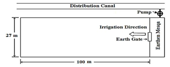
Fig. 3. General layout of earthen surface irrigation for field (No.3).
