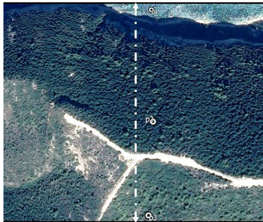
Fig. 6. Determining the mathematical coefficients needed to calculate the GSD.
