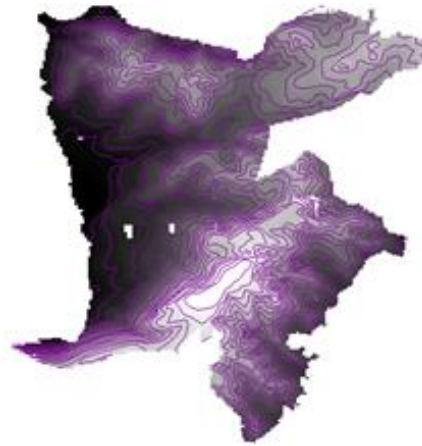
Fig. 10. The Digital Elevation Model (DEM) for the study area calculated from contour lines with elevations ranging from 0 to 350 m.
