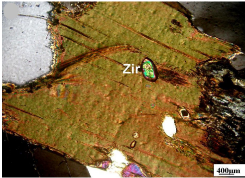
Fig.10: Photomicrograph of Batoga monzogranite showing biotite flakes enclosing zircon surrounded by the pleochroic haloes
