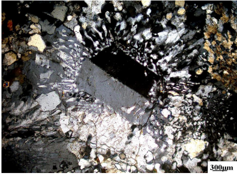
Fig.6: Photomicrograph of Batoga monzogranite showing Quartz intergrown with feldspar developing myrmekitic and graphic texture
