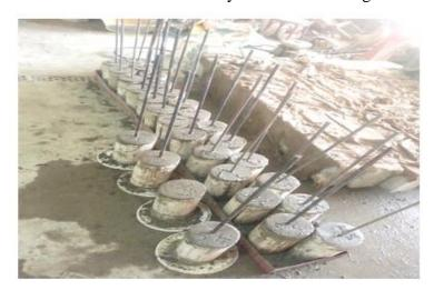
Fig. 5a. Compaction on concrete cubes and curing
