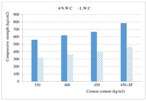
Fig.8. Effect of concrete type on the compressive strength of concrete cubes (350 kg/m<sup>3</sup>, 400 kg/m<sup>3</sup> and 450 kg/m<sup>3</sup> cement content).
