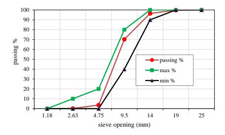
Fig. 4. Grading curve of lightweight aggregate
