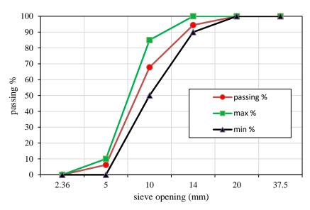
Fig. 2. Grading curve for crushed dolomite
