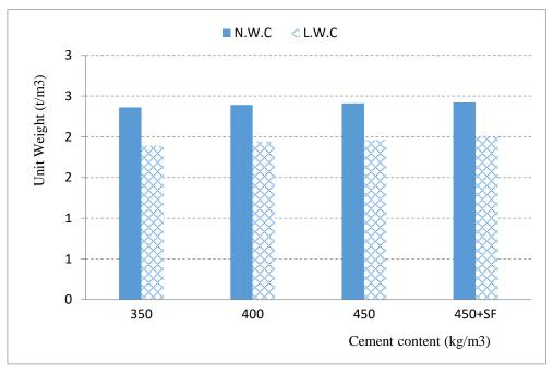
Fig. 9. Effect of concrete type on the unit weight of concrete cubes (350 kg/m<sup>3</sup>, 400 kg/m<sup>3</sup> and 450 kg/m<sup>3</sup> cement content.
