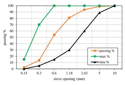
Fig. 1. Grading curve of sand
