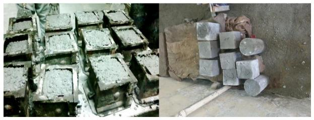
Fig. 5b. Compaction on concrete cubes and curing
