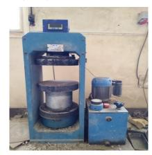
Fig. 7. Compression test
