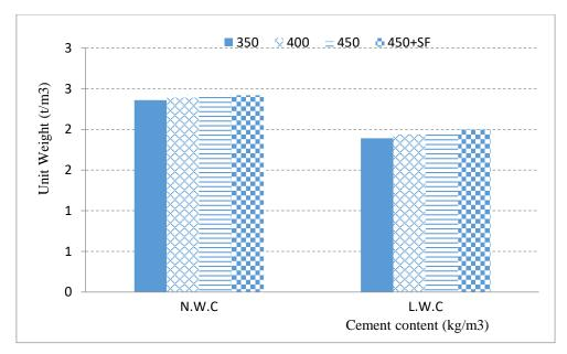
Fig. 11. Effect of cement content and silica fume on the unit weight of concrete cubes (350 kg/m<sup>3</sup>, 400 kg/m<sup>3</sup> and 450 kg/m<sup>3</sup> cement content.
