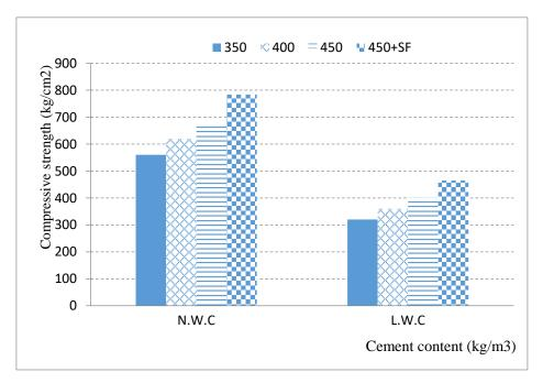
Fig. 10. Effect of cement content and silica fume on compressive strength of concrete cubes  $(350 \text{ kg/m}^3, 400 \text{ kg/m}^3 \text{ and } 450 \text{ kg/m}^3 \text{ cement content.}$
