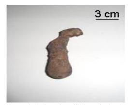
Fig.7: A single drop of metallic iron. The drop is rusted with brownish hydrated iron oxides
