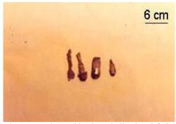
Fig.12: Four long white drops indicating definite melting and solidification of this material
