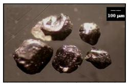
Fig. 30: Photomicrograph of cassiterite grains
