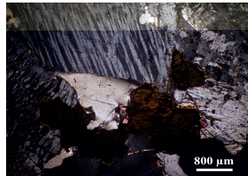
Fig.5: Photomicrograph of G. El Nekeiba qz-syenite showing string perthite associated with, arfvedsonite quartz and well-formed crystals of zircon, XPL.
