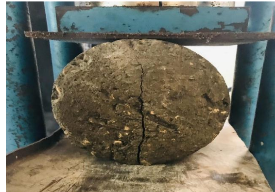
Figure 6: The failure mode of the concrete cylinder including PET particles in splitting tensile strength test
