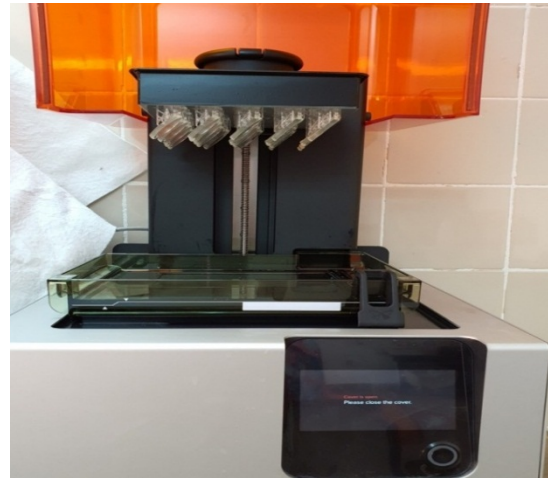
Fig.1: Dental LT Clear resin discs printed by FormLabs Form 2 machine
