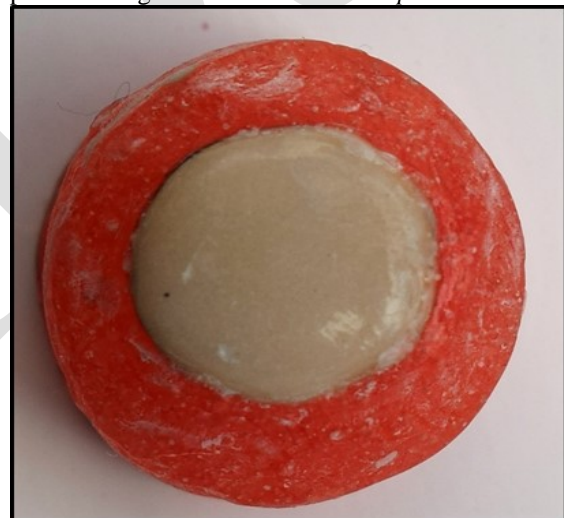
Fig. (1): Feldspathic porcelain disc embedded in self-cure acrylic resin cylinder.
