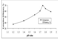
Fig. 1: Effect of pregnant leach liquor pH on the uranium extraction efficiency
