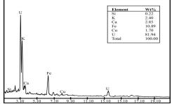
Fig 5: Scanning electron microscope EDX spectrum for the yellow cake end product
