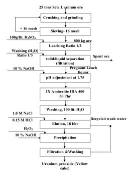
Fig. 6 : Flow diagram for the treatment of El Sela ore materials at Inshas Pilot Plant Unit
