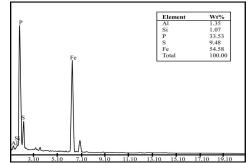
Fig. 2: SEM spectrum for precipitate from the pregnant leach liquor at pH 2
