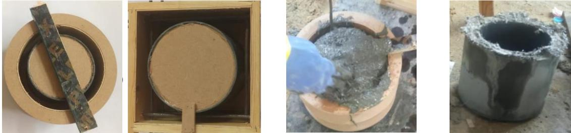
**Fig. 3: Fabrication of the prefabricated SHCC.**
