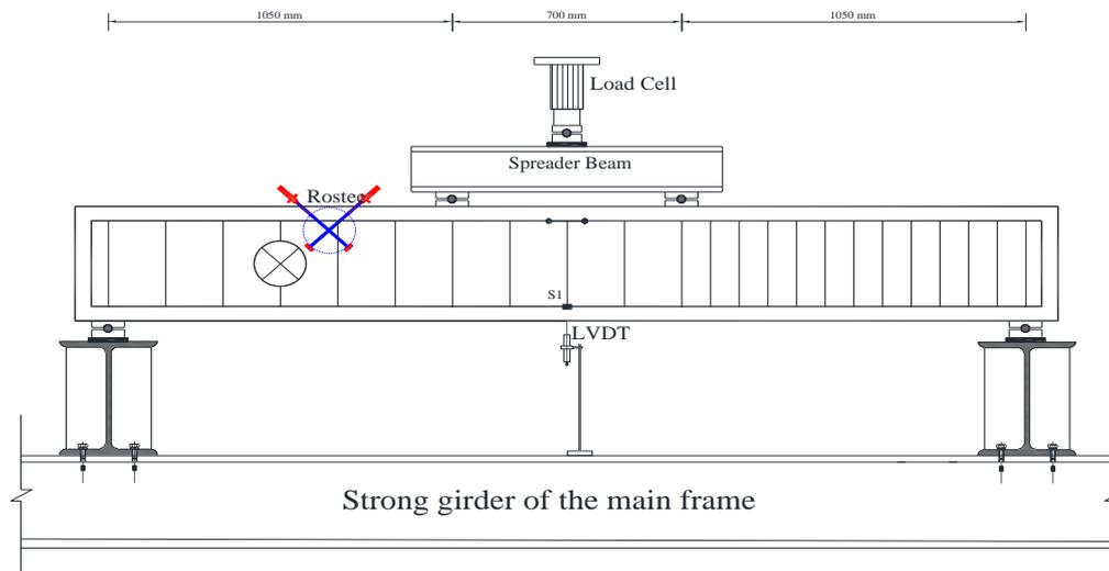
**Fig. 4: Test setup and instrumentations.**
